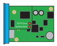
HTTP Error: Indicates internal errors in the configuration. For troubleshooting open the page http://xxx.xxx.xxx.xxx/diag in the device.
