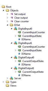
Here are the most important variables that can be used to retrieve the states of the IO end points:
