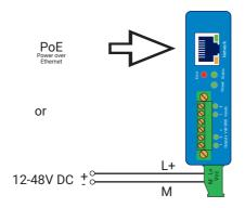
With a typical industrial power supply of 24V, the Web-IO draws approx. 100mA of current
