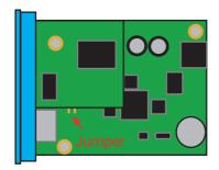
Close the jumper and power the Web-IO for approx. 30 seconds. The configuration has now been restored to its factory defaults.
