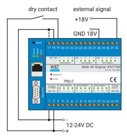
The galvanic isolation of the input groups allows the operation with different potentials. For example: Group 1 is connected to 18V and Group 2 to 24V.
