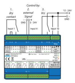
The galvanic isolation of the input groups allows the operation with different potentials. There are three variants:
