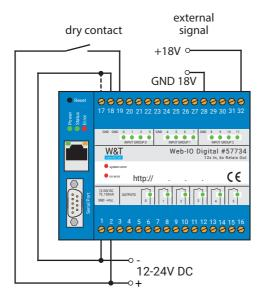
The galvanic isolation of the input groups allows the operation with different potentials. For example: Group 1 is connected to 18V and Group 2 to 24V.
