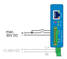
Positive voltages greater than 8V referenced to the -GND terminal are recognized as an ON signal and indicated as such by the corresponding LED.
