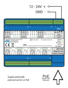
With a typical industrial power supply of 24V, the Web-IO draws approx. 100mA of current.
