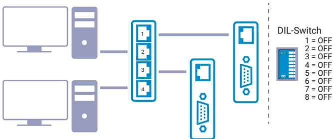
Each port automatically detects the transmission rate and whether data transmission should be in full or half duplex mode.
