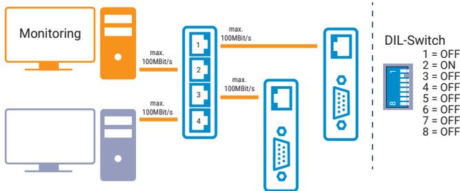
In the Monitoring mode, the complete data traffic handled by the switch is sent to the selected port. In this way, the data traffic of other network nodes can be read via network capture.
