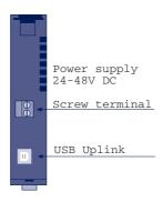
When connecting DC power supplies, please observe polarity as indicated on the screw terminal adapter:
