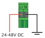
If you are using the W&T power supply, screw the power supply connector on to the screw terminal adapter:
