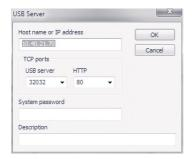
Enter the IP address or the host name of the desired USB-Server. The local TCP port on the USB-Server used for further communication defaults to 32032. If the UsbServerPort was reconfigured via Web Based Management on the USB-Server, the specified TCP-Port has to be changed accordingly in the Properties dialog box.
